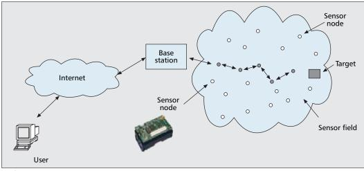
Figure 1. An example of a wireless sensor network.
