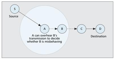
**Figure 2.** *Watchdog mechanism for MANETs.*
