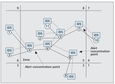
**Figure 3.** *The zone-based intrusion detection system for MANETs.*
